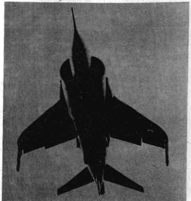
Fig.1.3 Kestrel. Note swept wing and extended span anhedral tailplane.
